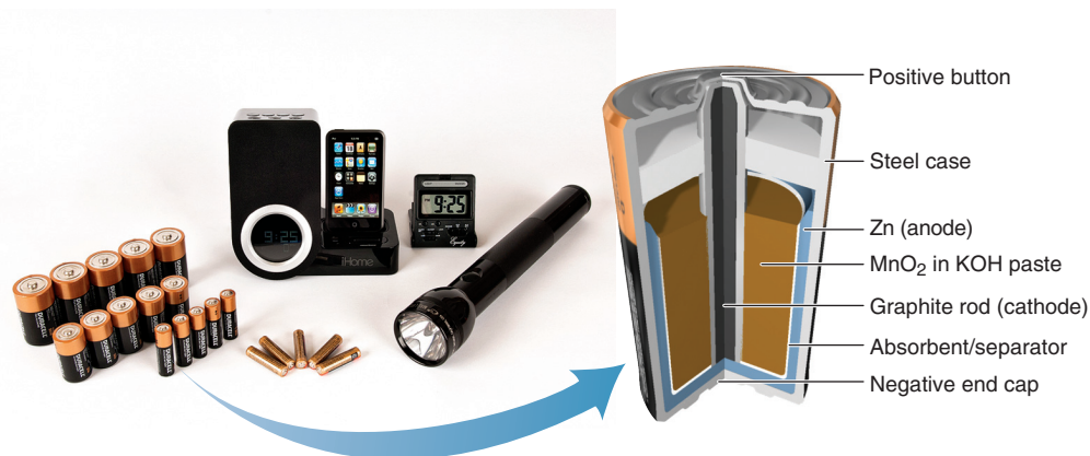
Figure 21.14 Alkaline battery.
