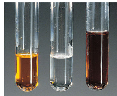
Dichromate ion ( left ) and iodide ion ( center ) form chromium(III) ion and solid iodine.
