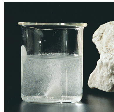
Figure 19.11 Test for the presence of a carbonate. When a carbonate mineral is treated with \text{HCl} , bubbles of \text{CO}_2 form.
