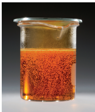
Figure 16.20 The catalyzed decomposition of \text{H}_2\text{O}_2 . A , A small amount of \text{NaBr} is added to a solution of \text{H}_2\text{O}_2 . B , Oxygen gas forms quickly as \text{Br}^-(aq) catalyzes the \text{H}_2\text{O}_2 decomposition; the reaction intermediate, \text{Br}_2 , turns the solution orange.
