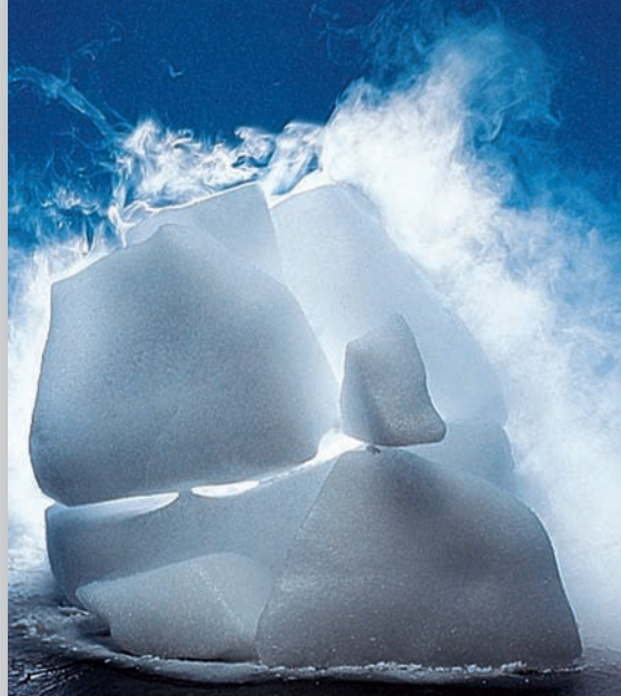
Under atmospheric conditions, solid carbon dioxide (dry ice) does not melt; it only sublimates.
