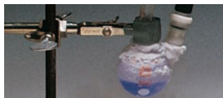
Liquid ozone below its boiling point ( -111.3^\circ\text{C} ). Ozone is a toxic, light-blue gas with a pungent odor.
