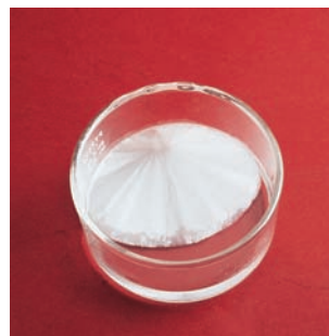
Figure 13.1 In a supersaturated sodium acetate solution (top), sodium acetate crystals rapidly form when a small seed crystal is added.
