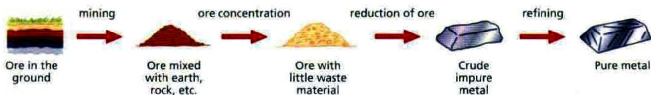
Fig. 14.15 The stages involved in obtaining metals from their ores
