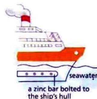
Fig 14.22 Rust prevention using a sacrificial metal
