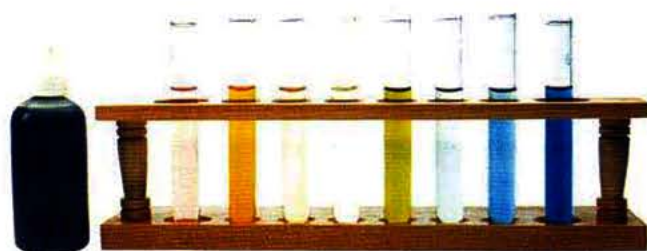
Fig. 11.12 The colour of Universal Indicator (paper or solution) is different in solutions of different pH.
