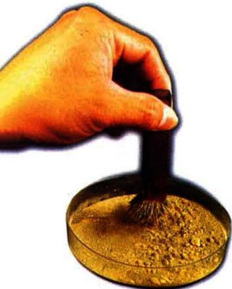
Using a magnet to separate iron from sulphur
