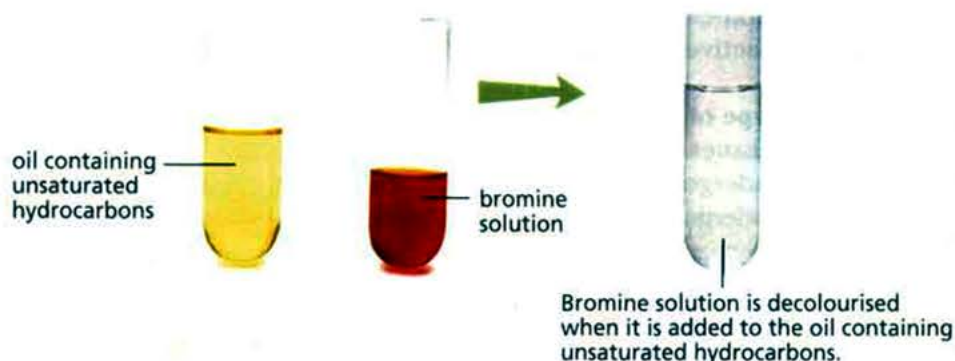
Fig. 23.5 Testing for the presence of unsaturated hydrocarbons
