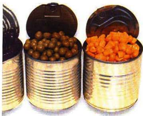
Food cans are tin-plated by electrolysis. Tin-plated food cans rust less easily.
