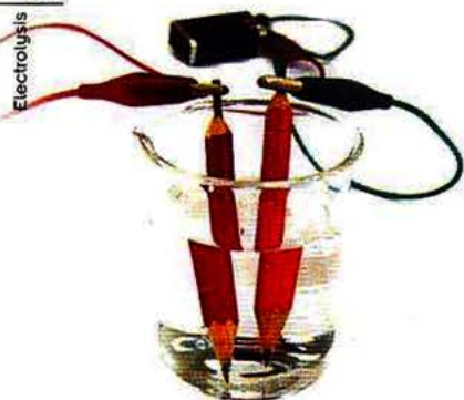
The lead in pencils contains graphite and can be used as inert electrodes in a simple set-up for electrolysis.
