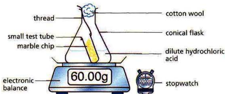
Fig. 18.4 An experiment to study the speed of reaction by measuring the mass at different time intervals
