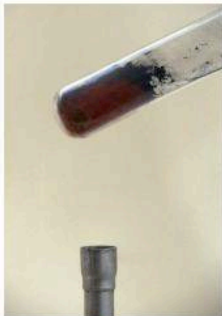
Figure 8.6 Notice the brown copper formed at the end of the reaction between carbon and copper(II) oxide.
