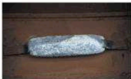
Figure 17.21 A sacrificial anode attached to a boat.
