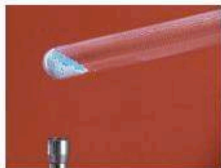
Figure 15.1 Copper(II) sulfate crystals are split into anhydrous copper(II) sulfate and water on gentle heating.
