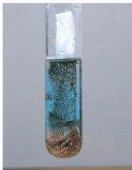
Figure 8.8 Zinc displaces copper from copper(II) sulfate solution.
