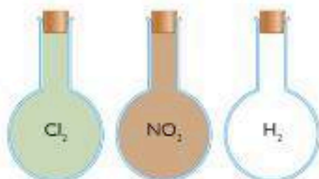
Figure 23.3 Three identical flasks containing different gases at the same temperature and pressure all contain equal numbers of molecules.
