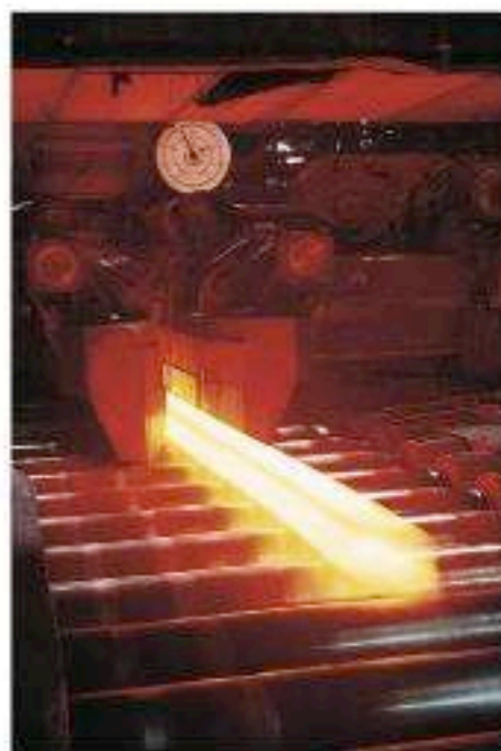
Figure 4.8 Steel being rolled into strips.
