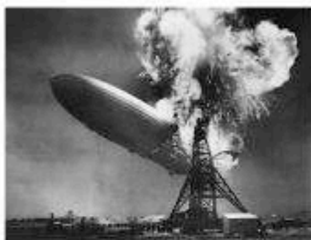
Figure 9.8 Because hydrogen is so light, it was used in airships – in 1937 the Hindenburg caught fire and 36 people were killed, most of them by jumping from the airship.
