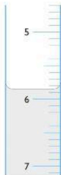
Figure A2 Measuring from the bottom of the meniscus.
