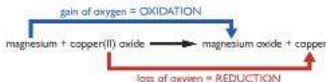
Figure 8.7 Magnesium reacting with copper(II) oxide.
