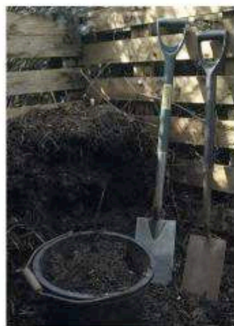
Figure 17.18 A mild steel spade tarnishes – a stainless steel one doesn't.
