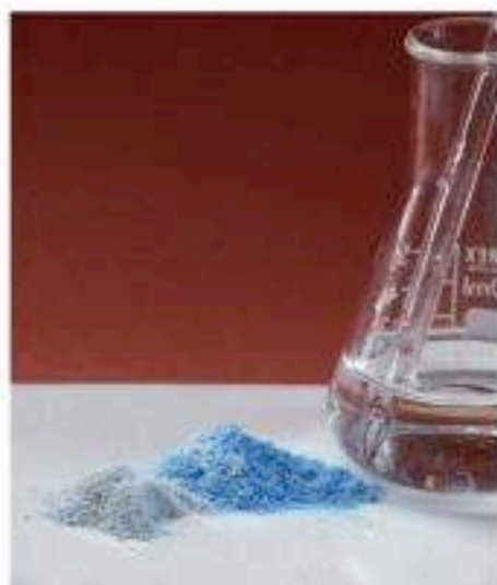
Figure 11.11 Testing for water with anhydrous copper(II) sulfate.
