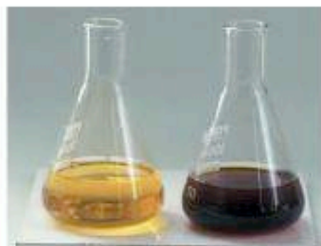
Figure 12.19 Bromine and iodine displaced from potassium bromide and potassium iodide solutions.
